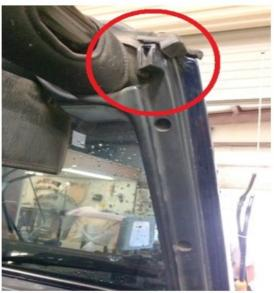
Figure 6 "Bent A-Pillar"
