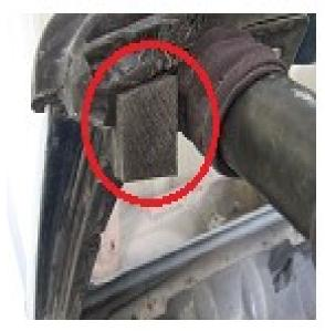
Figure 5 "Top to A-Pillar Gasket"
