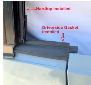
Figure 4 After Installation of the Tailgate Gasket and And Hardtop(driver's side view)
