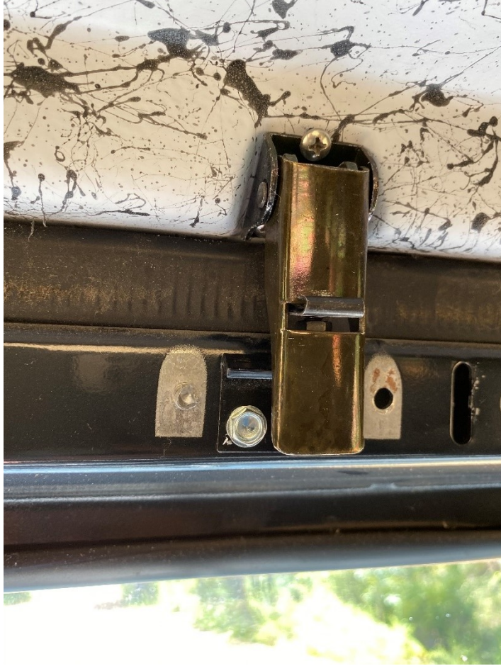
The center OEM tie down is replaced for Bull Dawgs install. Bull Dawg did supply a piece of trim to cover this. Pictured below
