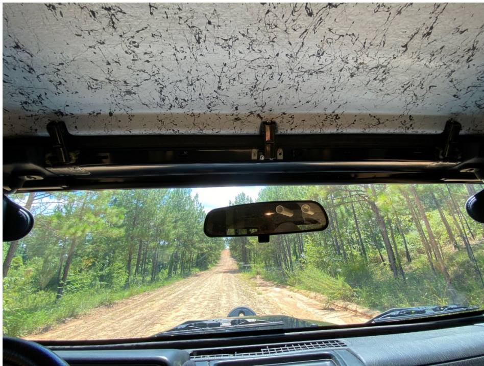
Here you can also see the three attachment cams at the windshield. These and the thumbscrews need adjustment within a few hours of install as the weather seal settles. Also, I had to flip my mirror right side up. How strange.
