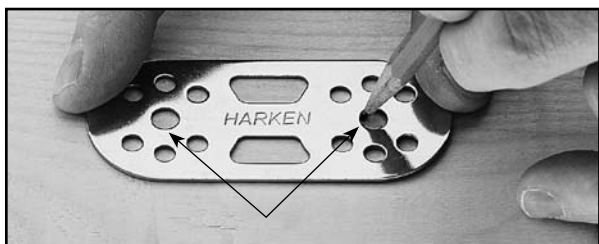
DIAGRAM 12. Center Rope Organizer Plate (K) between the two Pigtail Lag Screws (B) on front mounting board. Use as template to mark center holes.
