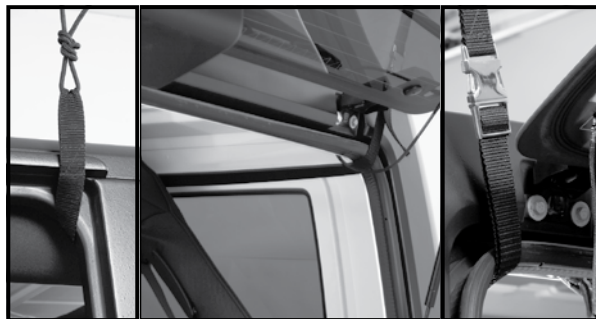
DIAGRAM 23. Run straps lengthwise from front door to rear tailgate between top and rollbar.
