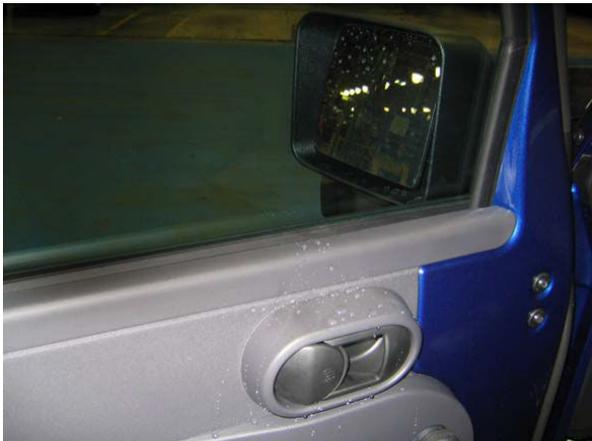
Figure 1: This repair procedure is applicable when water is evident on the door trim panel
