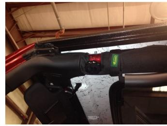
Figure 13 – “Properly Installed Knob/bolt”
