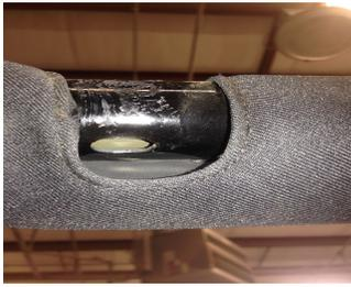
Figure 11 – “Hole in Roll-Bar”
