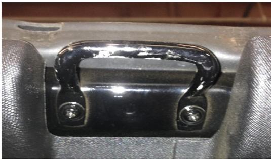
**Figure 5 – Factory Installed Footman Loops**
